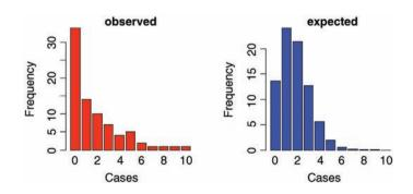
The distributions are very different: the mode of the observed data is zero, but the mode of the Poisson with the same mean is 1; the observed data contained examples of 8, 9 and 10 cases, but these would be highly unlikely under a Poisson process. We would say that the observed data are highly *aggregated*; they have a variance–mean ratio of nearly 3 (the Poisson, of course, has a variance–mean ratio of 1):
