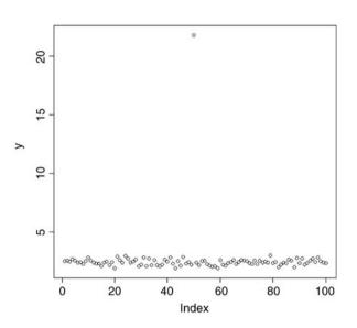
One data point sticks out like a sore thumb. We need to go back to the lab notebook and check what has happened. It is useful to know what line of the dataframe contains the unusually large value of y. This is easy to work out using the which function. Inspection of the plot shows that our questionable data point is the only one larger than 10, so we can use the which function like this:
