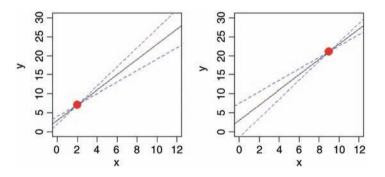
Confidence in predictions made with linear regression declines with the square of the distance between the mean value of x and the value of x at which the prediction is to be made (i.e. with  $(x - \bar{x})^2$ ). Thus, when the origin of the graph is a long way from the mean value of x, the standard error of the intercept will be large, and vice versa.
