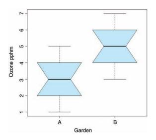
Because *the notches of two plots do not overlap*, we conclude that the medians are significantly different at the 5% level. Note that the variability is similar in both gardens (both in terms of the range – the length of the whiskers – and the interquartile range – the size of the boxes).
