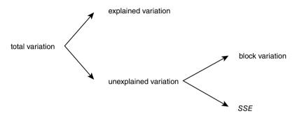
The idea of good experimental design is to make *SSE* as small as possible, and blocking is the most effective way to bring this about.
