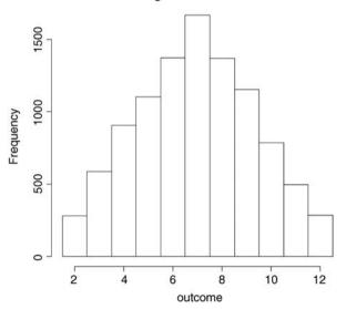
Note the trick of specifying the breakpoints to be offset by 0.5 in order to get the correct labels in the centre of the relevant bars.
