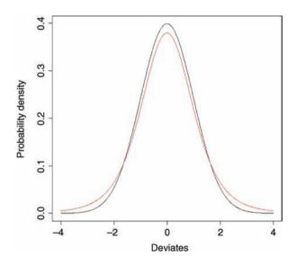
The difference between the normal (black line) and Student's *t* distributions (red line) is that the *t* distribution has 'fatter tails'. This means that extreme values are more likely with a *t* distribution than with a normal, and the confidence intervals are correspondingly broader. So instead of a 95% interval of  $\pm 1.96$  with a normal distribution we should have a 95% interval of  $\pm 2.57$  for a Student's *t* distribution with just 5 degrees of freedom:
