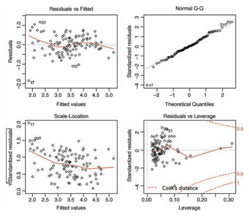
This shows that the variance and normality are now reasonably well behaved, so we can stop at this point. We have found the minimal adequate model. Our initial impressions from the tree model (no interactions) and the generalized additive model (a good deal of curvature) have been borne out by the statistical modelling.
