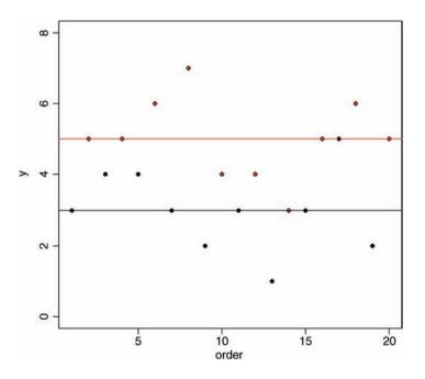
Now it is clear that the mean ozone concentration in garden B (red) is substantially higher than in garden A. The aim of ANOVA is to determine whether it is significantly higher, or whether this kind of difference could come about by chance alone, when the mean ozone concentrations in the two gardens were really the same.
