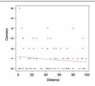
The red fitted line is curved, but very shallow. The trend is not significant (p > 0.18). Once you have understood the relationship between the linear predictor, the link function and the predicted count data, y, you can speed up the curve drawing with the predict function, because you can specify type="response", which carries out the backtransformation automatically:
