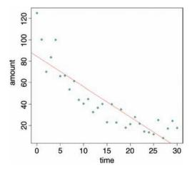
This draws attention to the pronounced curvature in the data. Most of the residuals at low values of time are positive, most of the residuals for intermediate values of time are negative, and most of the residuals at high values of time are positive. This is clearly *not* a good model for these data.
