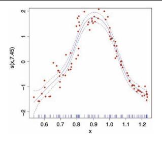
The y axis is labelled s(x, 7.45) which is interpreted as saying that the smoothed function of x shown by the solid blue curve ('the non-parametric smoother') involves the equivalent of 7.45 degrees of freedom (remember that a straight line would use 2 d.f.: the intercept and the slope). The dotted lines show the confidence interval for the location of the smoothed function of x. On the x axis you see a rug plot, showing where the x points on the graph are located.
