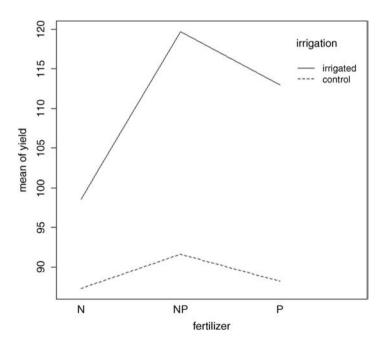
Irrigation increases yield proportionately more on the P-fertilized plots than on the N-fertilized plots. The irrigation:density interaction is more complicated:
