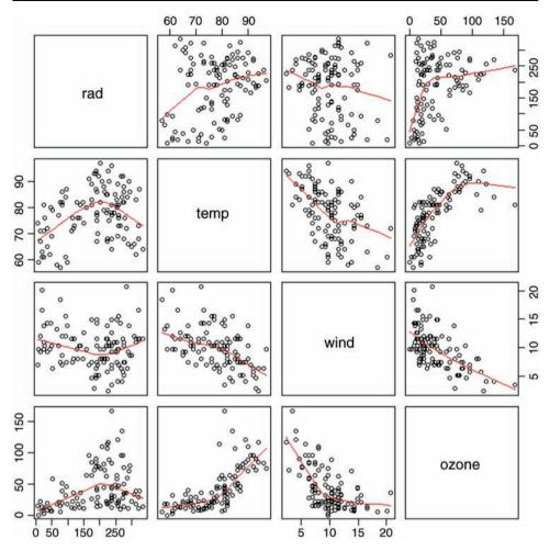
The response variable, ozone concentration, is shown on the y axis of the bottom row of panels: there is a strong negative relationship with wind speed, a positive correlation with temperature and a rather unclear, but possibly humped relationship with radiation.
