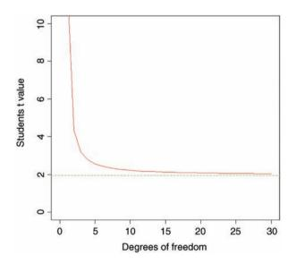
The importance of using Student's t rather than the normal is relatively slight until the degrees of freedom fall below about 10 (above which the critical value is roughly 2), and then it increases dramatically below about 5 degrees of freedom. For samples with more
